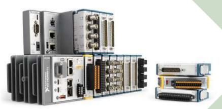
CompactDAQ (cDAQ) is a modular, PC based, data-acquisition hardware platform from National Instruments. In a CompactDAQ system, a chassis is connected to your PC through USB or Ethernet, and then populated with one or more conditioned I/O modules that provide direct sensor connectivity. You can synchronize the CompactDAQ Chassis to create a distributed system. CompactDAQ Controller variants are available that run a Windows or real-time OS for stand-alone operation.
