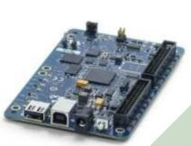
NI myRIO places dual-core ARM® Cortex<sup>™</sup>-A9 real-time processing and Xilinx FPGA customizable I/O into the hands of students. With its onboard devices, seamless software experience, and library of course-ware and tutorials, NI myRIO provides an affordable tool that students can use to do real engineering in one semester.
