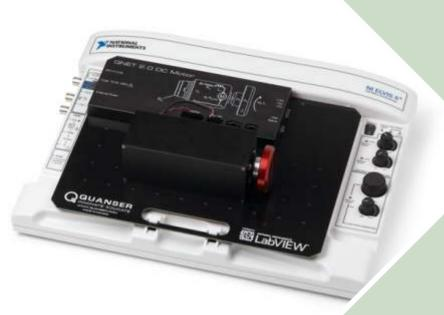
The QNET Mechatronic Actuators board is an ideal tool to introduce hands-on a variety of actuators, and demonstrate their advantages, interfacing and operation, as well as design considerations and limitations. This application board has been developed for education to facilitate hands-on, active learning of the common types of actuators used in mechatronic systems.
