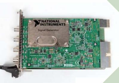
PXI-5402 is a 14-bit 20 MHz Arbitrary Function Generator device which has capability of 100 MS/s that feature up to 14 bits of resolution and 32 kB of on board memory for arbitrary function generation in a compact, 1-slot 3U PXI module.
