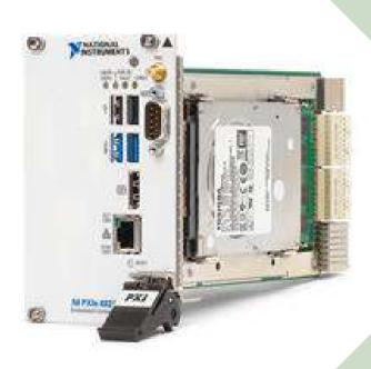
PXI Express/CompactPCI Express embedded controller is a high-performance PXI Express/CompactPCI Express-compatible system controller.
